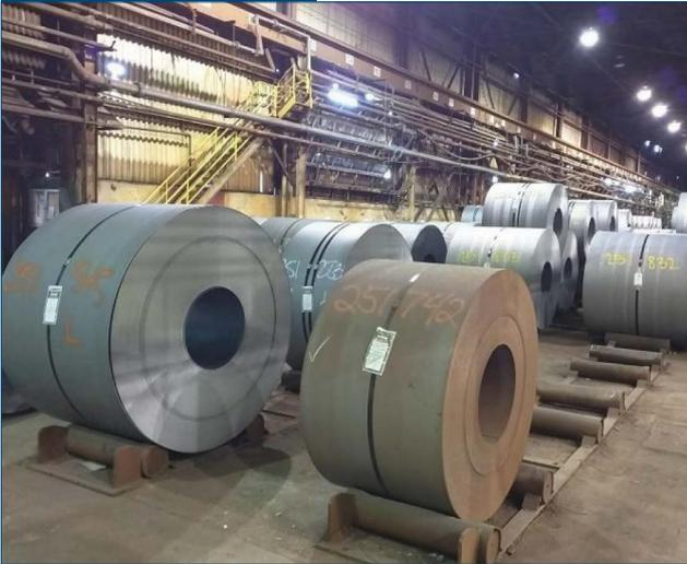
*Cold-rolled coils in a warehouse.*
