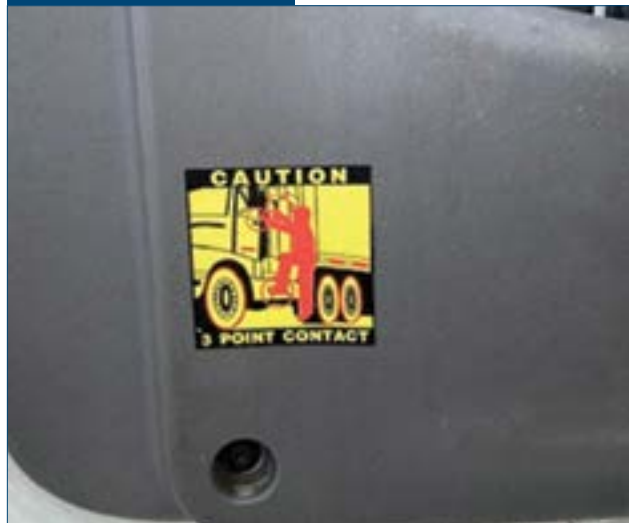
Stickers that were applied to areas where the drivers are commonly climbing to remind them of this key safety step.
