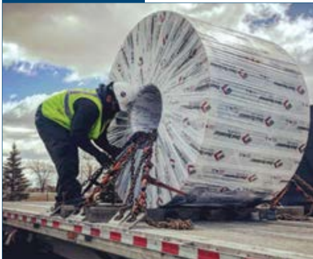
Flatbed load securement presents many tripping hazards.
