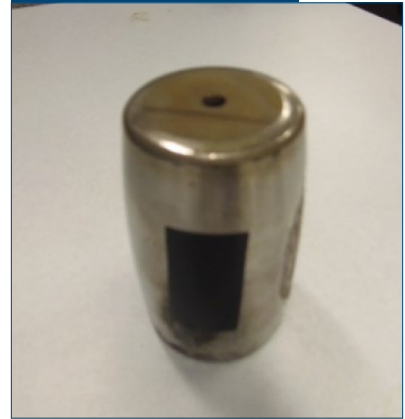
A roller element that contains both emissive and reflective surfaces that was heated to 115°F.
