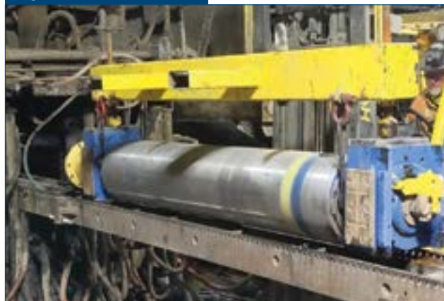
Roll spreader bar and forklift setting a roll.
