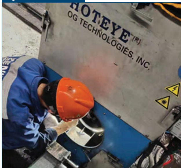
Exposed optics in regular cleaning.
