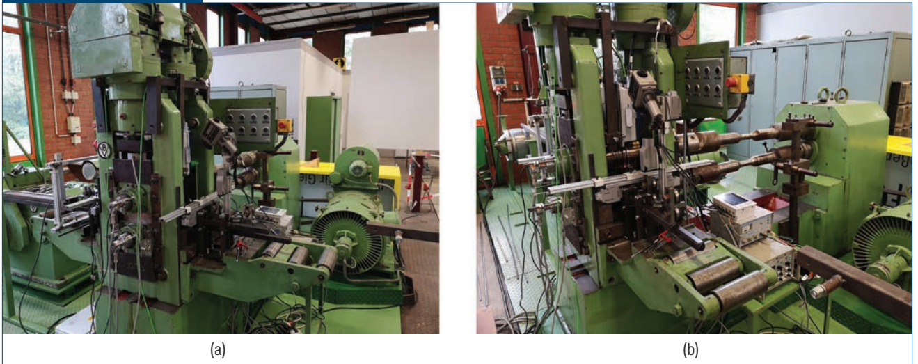
Laboratory rolling mill at the metal forming lab of UDE: operator side view (a) and entry side view (b).
