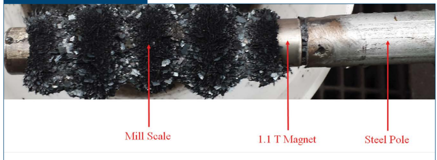
Mill scale recovered by the 1.1T magnet separator mounted on a carbon steel pole.
