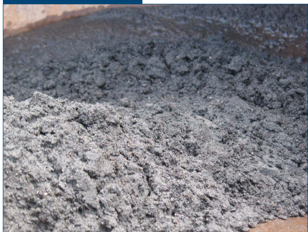
Separated grit discharged from the integrated dynamic separator.
